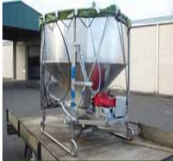
Alloy bucket with alloy and stainless steel components
